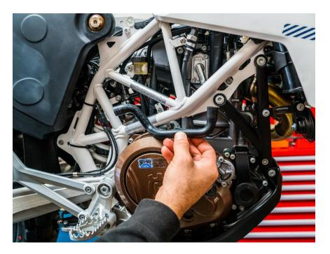
8. Remove the bolts and SAS plate and install the Rottweiler 'R' block off plate using the same 6mm bolts.
