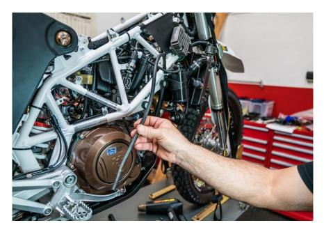
15. Identify the hose traveling from the rear fuel tank to the canister and unplug it from the canister.16. Remove the valve hose and canister from its mount.
