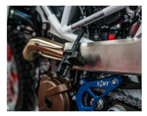
22. Insert the dongle into the harness plug that went to this valve.
