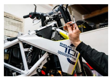
2. Locate the SAS valve (Shown below and cut both zip ties on both hoses)
