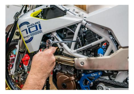
26. Replace the nipple with the small 6mm screw and copper washer.
