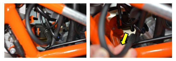
12. Pull the thicker of the two lines at the canister through the frame and out. You may have to rotate the outer coil stick to allow the line to pass through behind it.
