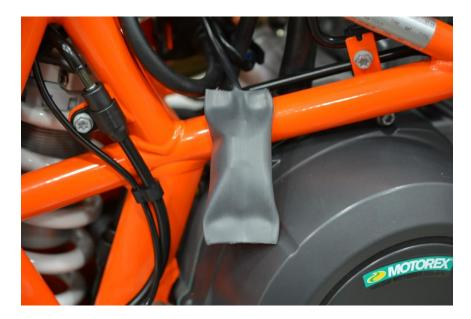
10. Zip tie the sealed plug into as safe place inside the frame.
