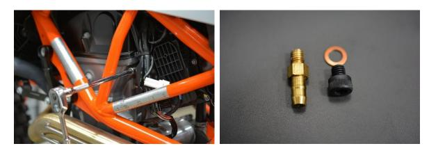
23. (5mm HEX) Replace the nipple with the small 6mm screw and copper washer.
