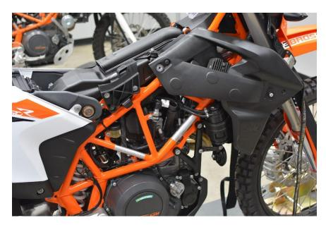
2. (T30/20 TORX) Remove the right-side inner panel. The GREEN circle notes a pin that can be released by hand.
