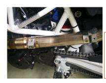
8) **701** Install the pipe clamp and bracket for the front heat shield mount leaving it slightly loose so it can be adjusted to the heat shield making sure the screw for tightening the bracket is on the bottom.
