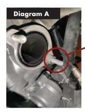
Note: For the **KTM 690** ensure the spacer is installed on the bottom flange stud see Diagram A
