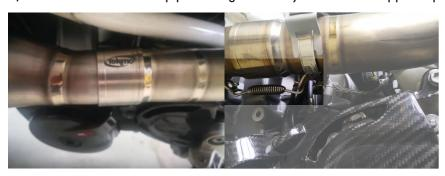
4) Install the rear mounting bracket using the aluminum spacer and the longer bolt supplied with your Tekmo header need to be used, the aluminum spacer should go on the bottom, the bolt should be left loose.
