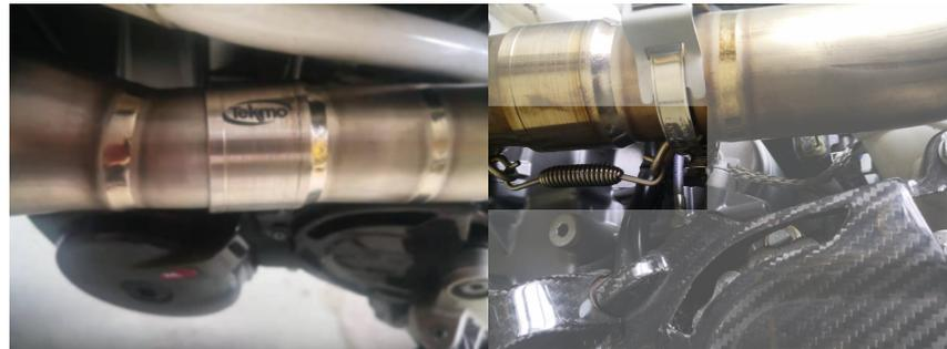
4) Install the rear mounting bracket using the aluminum spacer and the longer bolt supplied with your Tekmo header need to be used, the aluminum spacer should go on the bottom, the bolt should be left loose.
