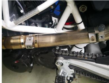
8) **701** Install the pipe clamp and bracket for the front heat shield mount leaving it slightly loose so it can be adjusted to the heat shield making sure the screw for tightening the bracket is on the bottom.
