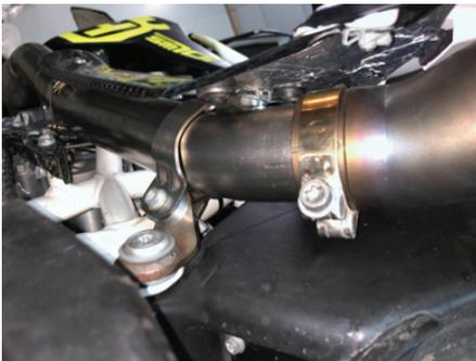
7) Tighten up the rear muffler to header pipe clamp.
