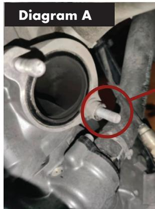
Note: For the **KTM 690** ensure the spacer is installed on the bottom flange stud see Diagram A
